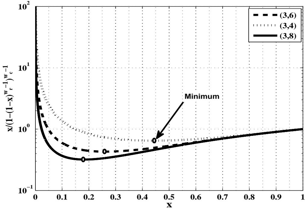
Figure 6.2: Supremum of can be found by minimizing  $\frac{x}{\lambda(1-\rho(1-x))}$ . Shown are there examples for three different regular LDPC codes.
